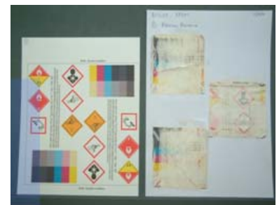
Print failure after abrasion
