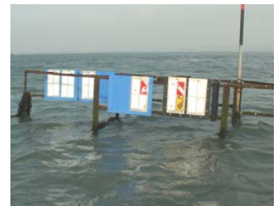
Pira marine immersion test rig
