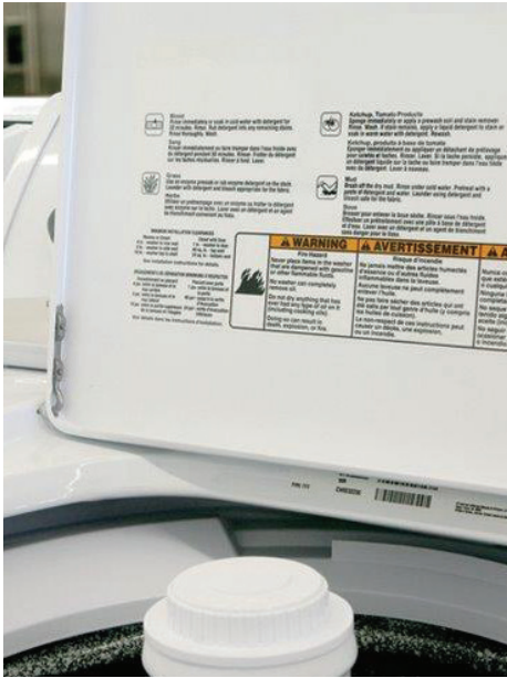
UL labels specific to indoor use products must withstand 72 hours at 23+2 degrees Celsius, 50+5%RH; water immersion for 48 hours at 23 degrees Celsius; and, 10 days in an air oven with temperatures at 20 to 30 degrees Celsius higher than rating temperature
