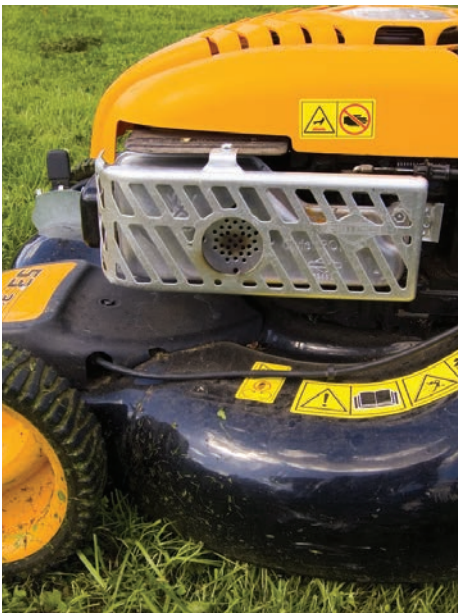
UL labels specific to outdoor use products must withstand 7 hours in a low temperature cold box at a temperature of -23 degrees Celsius or lower; 750-hour UV and water exposure; and various immersions
